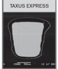
Strut thickness: 132 μm Coating thickness: 19.6 μm
