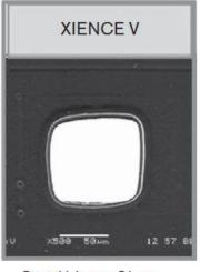
Strut thickness: 81 μm Coating thickness: 7.8 μm
