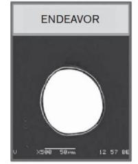
Strut thickness: 91 μm Coating thickness: 4.8 μm
