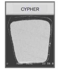
Strut thickness: 140 μm Coating thickness: 12.6 μm
