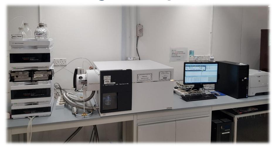
Figure 3: UHPLC Triple Quad LCMS System
